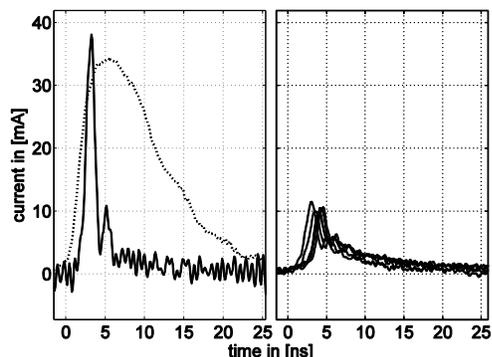
Figure 7. Left: First-PD with minimum X-ray dose at  $E=1.3 \text{ kV/mm}$ . Electrical pulse and PMT pulse (dotted line). The electrical pulse has a rise-time of 1.3 ns pulse and pulse-width 1.4 ns. The PMT pulse has a rise-time 2.9 ns and pulse-width of 10.6 ns. Right: 5 subsequent-PDs (PD number 2 to number 6) with minimum X-ray dose. Average rise-time of subsequent pulses is 2.3 ns and pulse-width 2.3 ns.
