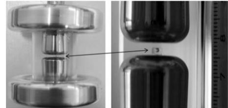
Figure 2. Left: sample with shield electrodes (as used in PRXPD); Right: design of the transparent epoxy samples with rod-rod geometry electrodes and the single spherical void (1 mm diameter) between.
