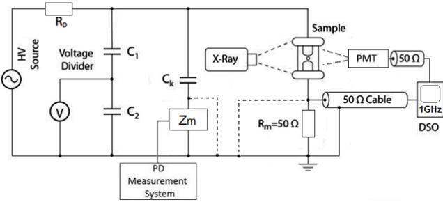
Figure 3. Principle diagram of the PXIPD circuit. By shortening of either  $Z_m$  or  $R_m$  it can be used as PRXPD or TRXPD setup. For TRXPD measurements the  $C_K$  is replaced by the self-built  $C_K$  shown in Figure 4.
