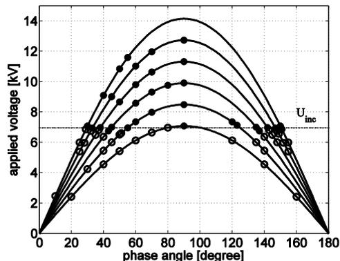
Figure 6. Voltage on sample vs. phase angle instant of single X-ray pulse application. Each point in the graph represents a new TRXPD measurement. The full circles refer to a successful PD inception and the open ones give the voltage levels where no PD inception occurs.
