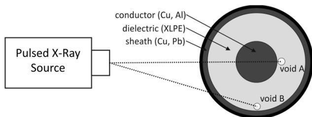
Figure 8. Schematic (simplified) representation of a solid insulated cable with two defects [17].
