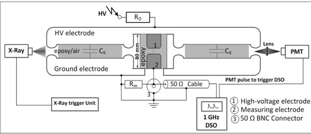
Figure 4. Diagram of the TRXPD measurement circuit and the PMT: Cross section of the “short discharge path ring coupling capacitor”  $C_K$  with the sample in the middle. The epoxy ring with the high voltage electrode and ground electrode builds the coupling capacitor.
