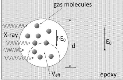
Figure 1. X-ray application to a void in a solid insulator
