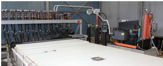
Figure 1. Partial view over some of the ageing components of the ICAAS system and the cable samples
